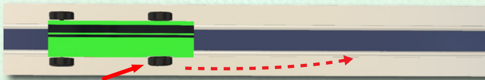
Front wheel set to slightly steer the car into the center rail.
